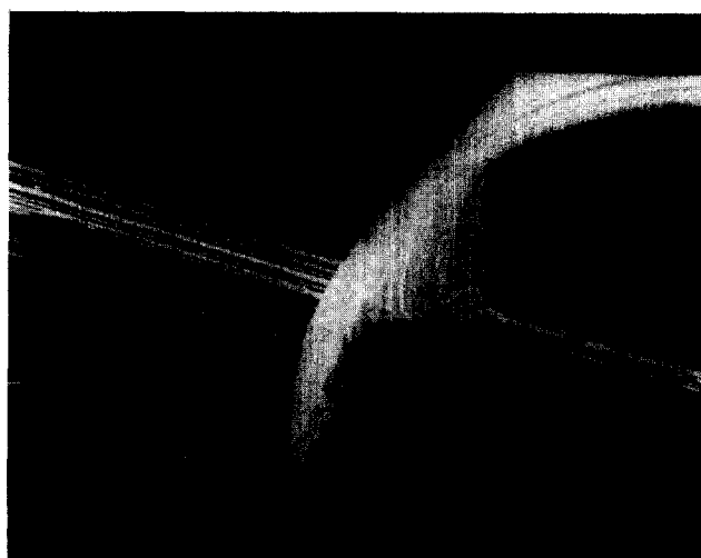
Figure 5 Sheath of fibrils beneath skin peeled from Kevlar 49 fibre, bent as shown. Buckling of fibrils in high-curvature region is evident
