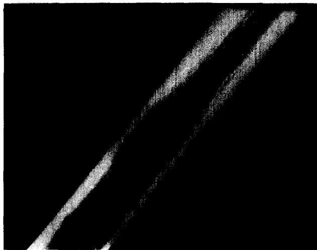
Figure 11 Coated PBO fibre cycled to 430°C in vacuo . Differential radial thermal expansion cracked coating. Good adhesion prevents spalling. Despite cracking, radial coefficient of thermal expansion of coated fibre remained below that of uncoated fibre
